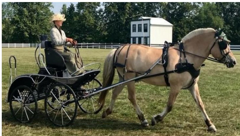
Closed end shafts on a marathon vehicle keep the shafts from dropping if the singletree came off.
