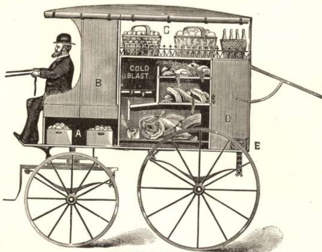
REFRIGERATOR WAGON. PLATE No. 48.—HALF-INCH SCALE.— Explanation on page 102.
